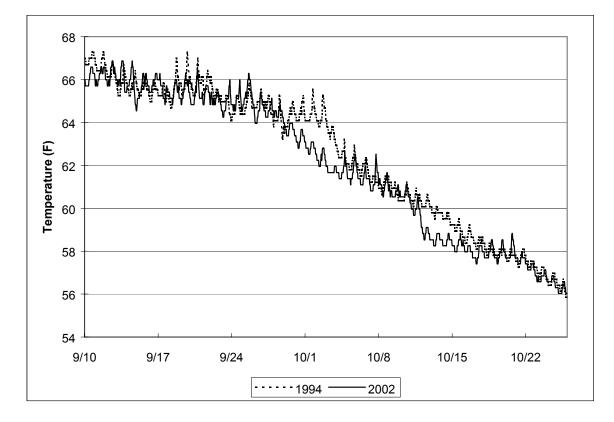
Figure 9. Iron Gate Dam hourly discharge temperatures (°F) for September 10 – October 25, 1994 and 2002.
