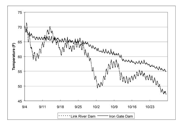
Figure 6. Hourly water temperatures measured at the Upper Klamath Lake discharge into Link River and Iron Gate Dam discharge temperatures, September 4 to October 29, 2002.
